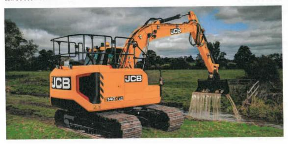
A safe working area of 1m should be left behind the counterweight. This adds up as:
