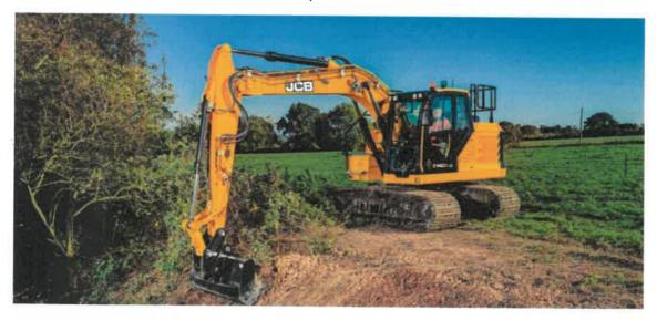
To operate safely the machine needs to be a minimum of 1.5m back from the edge of a pond or watercourse to ensure that there is no impact on the bank and a bank slip could potentially cause the machine to over-turn into the pond.
